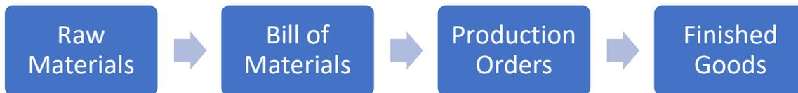
The production process starts with adding a production order and releasing it to production. Production order is the main document in the production process. It records the progress of the production process for each item produced. The production order is based on the bill of materials. Once the production work is done, the completion of the production order is reported and the finished goods/items are received into the warehouse.
